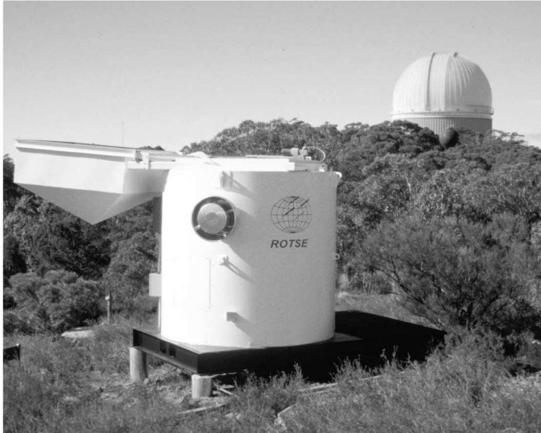
FIG. 3.—ROTSE-III telescope enclosure at the Siding Springs Observatory near Coonabarabran, Australia, with the hatch cover fully open. The telescope optics have not yet been installed. The 4 m Anglo-Australian telescope is in the background.
